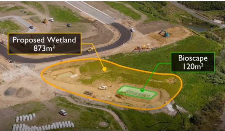
Ōmokoroa Filterra® Bioscape®: Catchment area: 3.25 hectares Bioscape® footprint: 120m²
