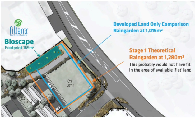
Lake Tekapo Filterra® Bioscape®: Catchment area: 5.1 hectares Bioscape® footprint: 165m²
